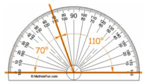
Make sure that the vertex/centre (hole or indentation) of the protractor is exactly over where the two lines meet.
